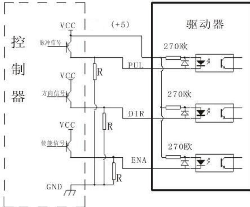
Fig. 2 Input port circuit ( Negative connection)
