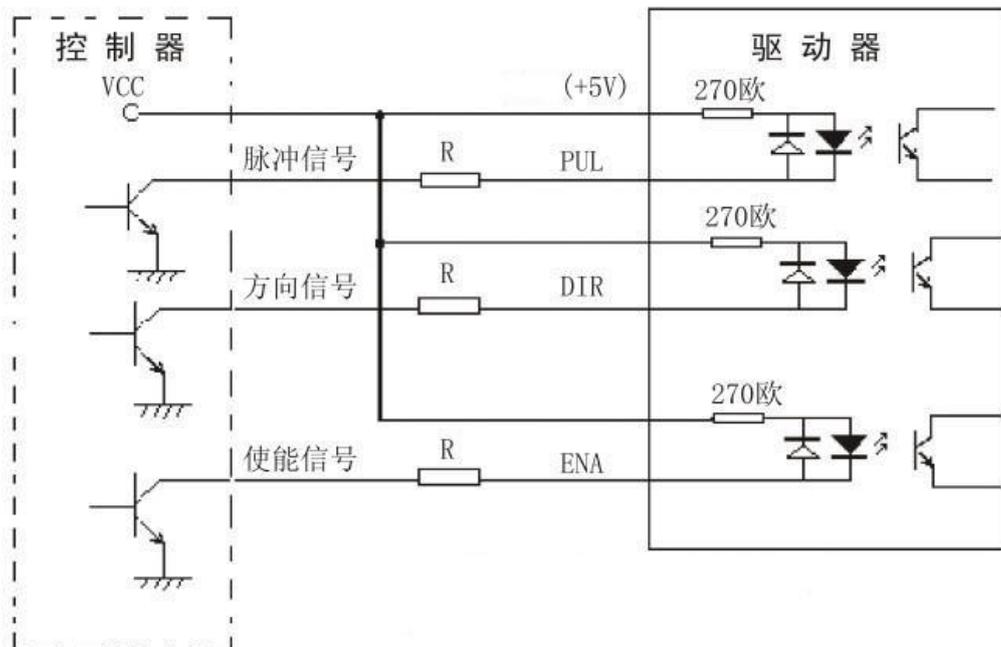
Fig 1. Input port circuit (Positive connection)
